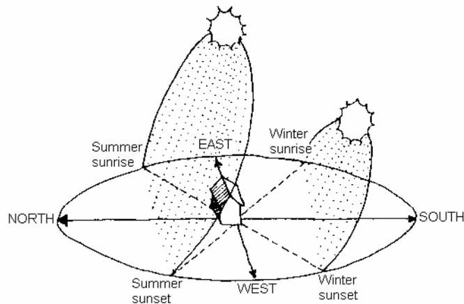
**Figure A.3.** Paths of the sun on winter and summer solstices (Sand 1991). Summer heat gain is primarily through east- and west-facing windows and walls. The roof receives most irradiance, but insulated attics reduce heat gain to living spaces. The winter sun, at a lower angle, strikes the south-facing surfaces.
